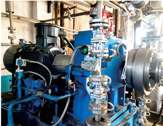
甲醇精馏装置用甲醇压缩机 Methanol compressor for methanol distillation unit
