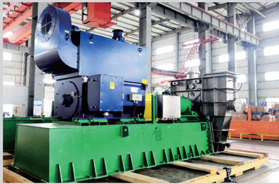
高纯晶硅污水处理 两台串联 The sewage treatment device in a polysilicon project Two stages connected in series
