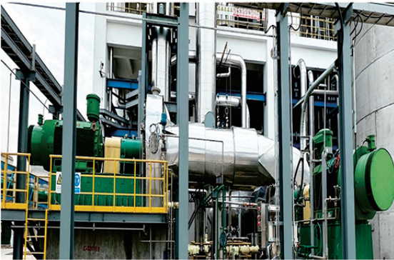
己内酰胺聚合装置 两台串联 Caprolactam polymerization unit Two stages connected in series
