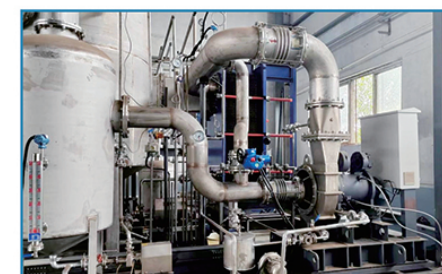
某饲料添加剂蒸发浓缩项目蒸汽压缩机 Steam compressor for a feed additive evaporation and concentration project
