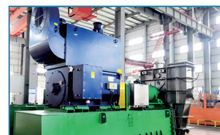
某高纯晶硅项目污水处理装置蒸汽压缩机 Steam compressor of the sewage treatment device in a polysilicon project
