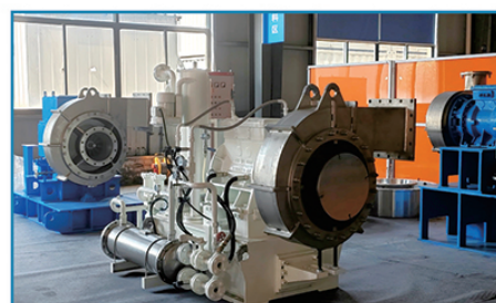
注射液低温浓缩用蒸汽压缩机 Steam compressor for low-temperature concentration of injectable liquid
