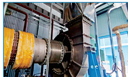
某制药废水蒸发结晶项目蒸汽压缩机 Pharmaceutical wastewater evaporation crystallisation project
