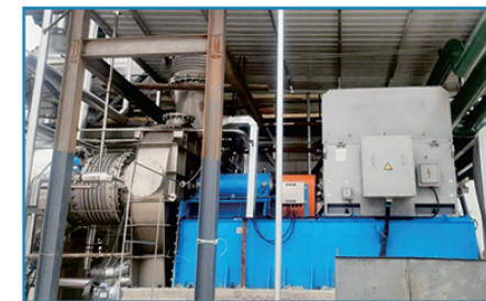
某番茄酱浓缩项目蒸汽压缩机 Steam compressor for a tomato sauce concentration project
