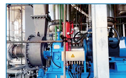
某三氯蔗糖（无糖可乐）蒸发结晶蒸汽压缩机 Evaporation crystallization of sucralose (sugar free cola)
