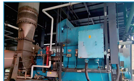
某锂电池生产废水处理项目 Steam compressor for the treatment of the wastewater in a lithium battery project 蒸发量：56 t/h Evaporation capacity: 56 t/h
