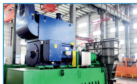
某高纯晶硅项目污水处理装置蒸汽压缩机 Steam compressor of the sewage treatment device in a polysilicon project 蒸发量：65.5 t/h+66.5 t/h Evaporation capacity: 65.5 t/h+66.5 t/h 两台串联 Two series connected
