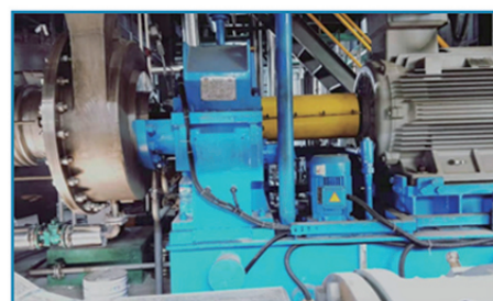
某三氯化铁蒸发结晶工艺蒸汽压缩机 High temperature rise steam compressor of ferric chloride evaporation and crystallization process of a fine chemical company
