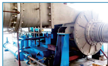
某螯合剂浓缩工艺蒸汽压缩机 High temperature rise steam compressor for the chelating agent concentration project of a chemical plant
