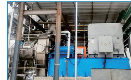
某番茄酱浓缩项目蒸汽压缩机 Steam compressor for a tomato sauce concentration project 蒸发量：50 t/h Evaporation capacity: 50 t/h
