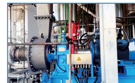
某三氯蔗糖（无糖可乐）蒸发结晶蒸汽压缩机 Evaporation crystallization of sucralose (sugar free cola) 蒸发量：8 t/h Evaporation capacity: 8 t/h
